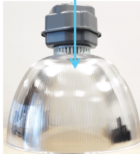
HID High-bay: 28,000LM/400W Circuit Box: D=200mm, Depth=200mm Reflector: D=590mm, Depth=310mm
